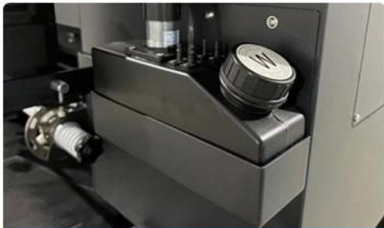
White ink stirring pump to prevent the precipitation of white ink and improve the printing effect.
