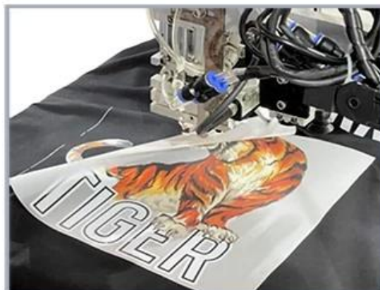
6. Robotic arm peels off the finished transfer film
