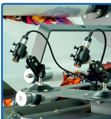
Laser Positioning System
