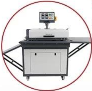
Outfeed - Adjustable Table Inclination
