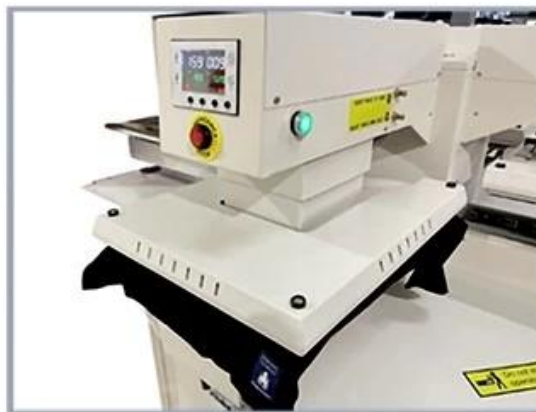
4. Heat platen is automatically pressed down for heating
