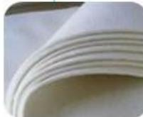
**Woollen felt:** The buffer between the two heating platens, ensures the flatness of the contact surface.
