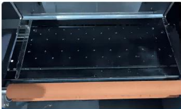
The vacuum adsorption platform ensures printing stability efficiently.
