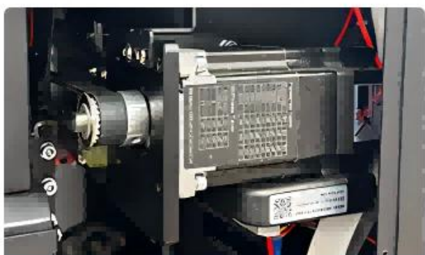
High-quality servo industrial motor drive system ensures the accuracy and stability of printing.
