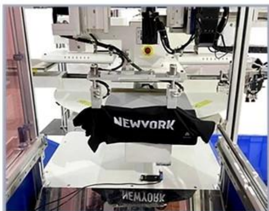
7. Automatically grabs the transferred T-shirts
