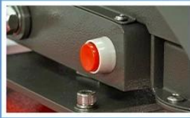
Emergency Release Button
