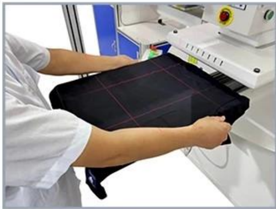
1. Place the T-shirt onto S4 automatic carousel heat press
