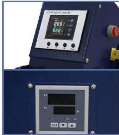
Two Independent Controllers for Accurate Printing
