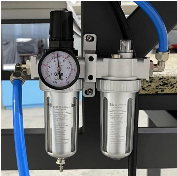
Air Filter System: the integrated air filter system provides improved air quality, protection for machinery, reduction of contamination, enhanced safety, and easy maintenance.
