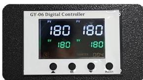
**Upgrade GY-06 Digital Controller.** This digital controller shows directly setting time, temperature and counter, and present time and temperature at the same time.
