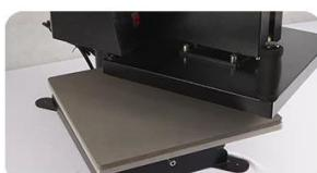
**Operator Safety:** Swing-away design not only enhances pressure but also contributes to operator safety by moving the heating element away from the work area during placement and removal of substrates.
