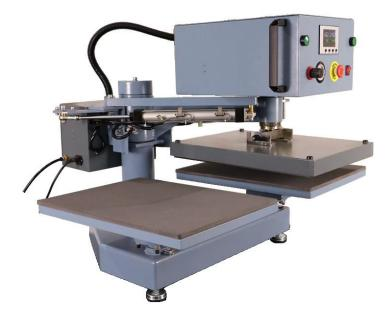
**Double Table Efficiency**: Equipped with a double table feature, allowing operators to prepare the next item for pressing while the first table is in use, optimizing workflow in high-volume production environments.
