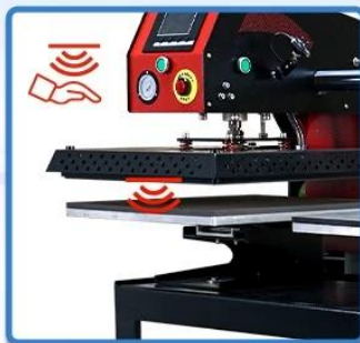
Built-in Sensor Hand-injury Prevention
