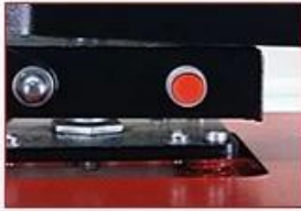
Manual Release Button For Emergency Issues
