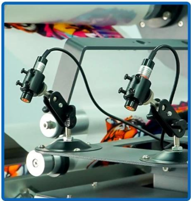
Laser Positioning System
