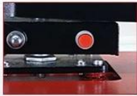
Manual Release Button For Emergency Issues
