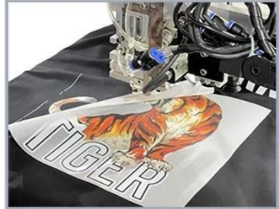
6. Robotic arm peels off the finished transfer film
