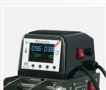
Controller for Upper Heater
