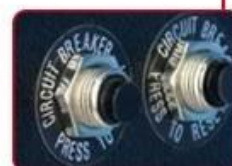
Back up circuit breaker
