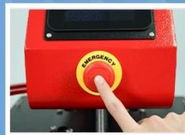
Emergency Stop for Safety
