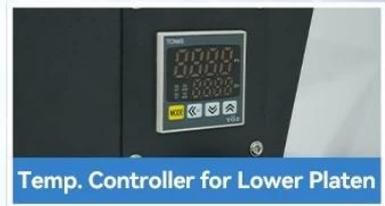
Temp. Controller for Lower Platen
