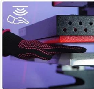
Built-in Sensor Hand-injury Prevention
