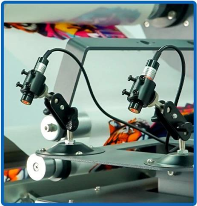
Laser Positioning System
