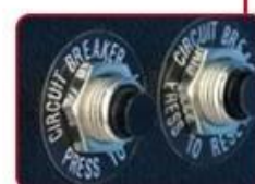
Back up circuit breaker
