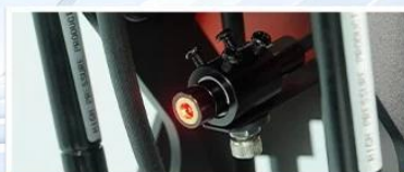
Laser Positioning System
