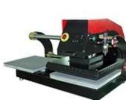
Pneumatic Double Location Shuttle Heat Press
