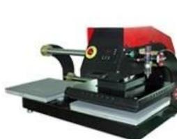
Pneumatic Double Location Shuttle Heat Press
