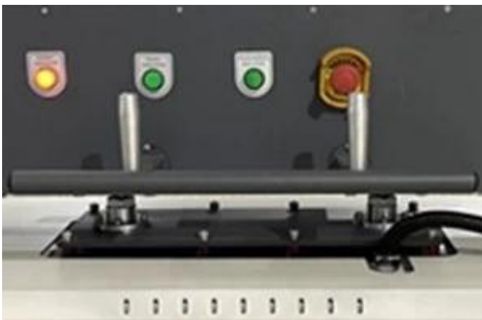
Safety Two-hand Control —this two-hand control ensures enhanced safety by requiring simultaneous activation of buttons with both hands. Prevents accidental operation, protects the operator from potential injuries.
