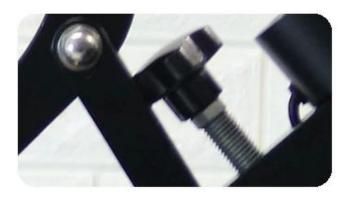
Pressure Adjust Knob: To adjust the pressure easily when sublimate items with different thicknesses.
