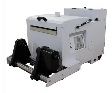
Even powder distribution: The auto powder shaking machine ensures that the DTF hot melt powder is evenly distributed on the DTF film, leading to high-quality prints with sharp edges and accurate colors.
