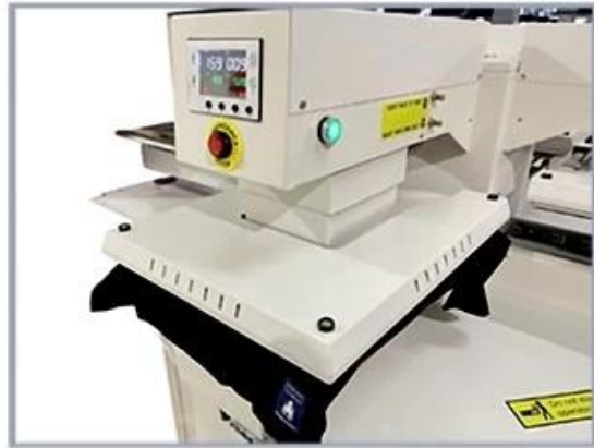
4. Heat platen is automatically pressed down for heating
