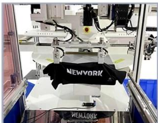
7. Automatically grabs the transferred T-shirts
