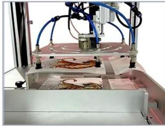
2. Mechanical arm grips the heat transfer material
