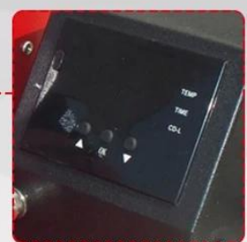
GY-04 Digital Time & Temperature Controller
