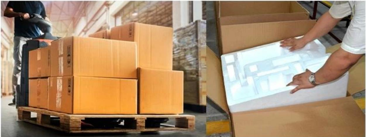
**Cardboard Box Packing:** Standard export boxes with internal cushioning of pearl cotton to ensure safe transportation of goods. Warning signs for proper box placement and waterproof bags inside.
