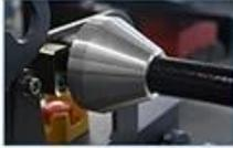
**Spring Loaded Take-up Mandrels:** No tools are required to load or remove media from the calender.
