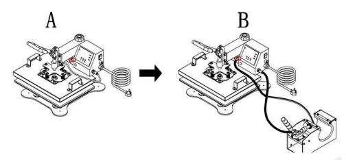
Disconnect the power connector of heat platen as the above picture shown.
