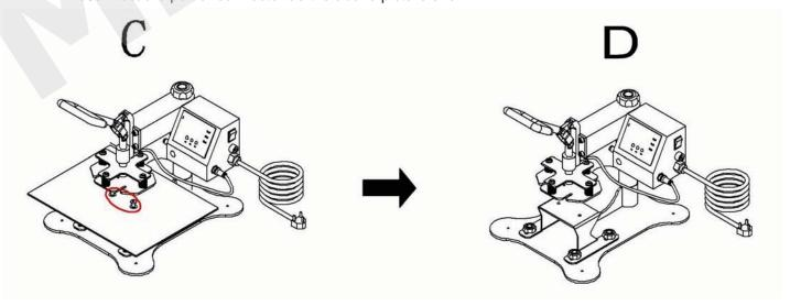
Remove the heat platen and under plate. Install the heat element as the above picture shown.
