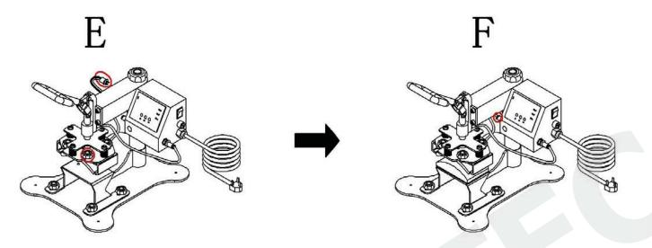
Tighten the screws of cap heat element, then connect the wire to the power connector.
