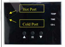
Note: There are two small port in front side of the digital display. If the real temperature is lower than digital controller shown, you can adjust the "hot port"; Clockwise to raise temperature; anticlockwise to reduce temperature.
