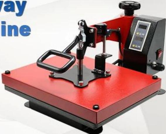
The image shows a red and black manual heat press machine. It features a large red platen at the base, a black frame, and a black handle on the left side. A control panel with a digital display and buttons is located on the right side. The machine is designed for heat pressing items like t-shirts and mugs.
