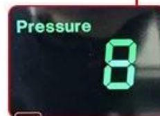
Internal pressure indicator in GY-08 controller
