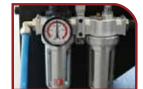
Air filter control the high pressure
