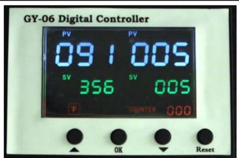
Press **OK** button to operating mode. Counter is "transfer cycle", from 0~999. Press "Reset" for 5 seconds to make the counter to be "0".
