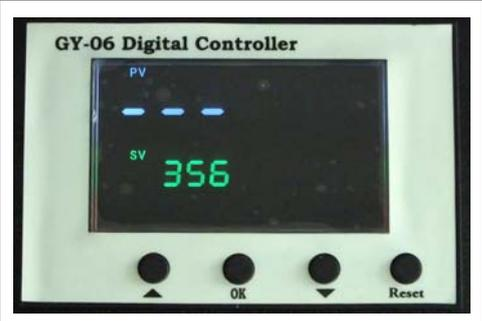
Press **OK** button, the temp
