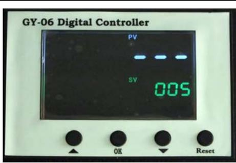
Press **OK** button after temperature setting and the time light is on. Select with arrows the time according to different transfer material.
