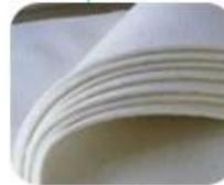
**Woolen felt:** The buffer between the two heating platens, ensures the flatness of the contact surface.
