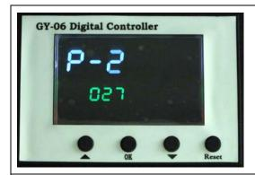
When SV and PV has a big difference, press  $\textcircled{\mathbb{R}}$  button for 5 seconds, and press  $\textcircled{\mathbb{R}}$  button again to adjust the temperature. If SV&PV has difference of 20 degrees, Press arrows " $\triangle$ " or " $\nabla$ " to set to 20.
