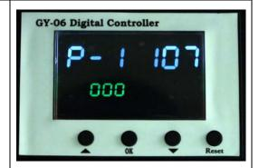
When the temperature shows on the display is not the same as actual temperature on heat platen, press button for 5 seconds to reset mode:
