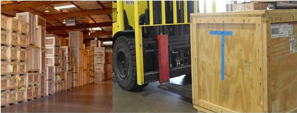
Wooden Crate Packing: For large machine, machine's feet are locked onto the crate to prevent movement during transportation, and the crate has forklift slots for easy customer transportation. The material is plywood, which avoids fumigation and reduces transportation costs.
