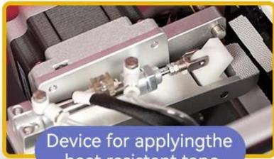
Device for applying the heat resistant tape
