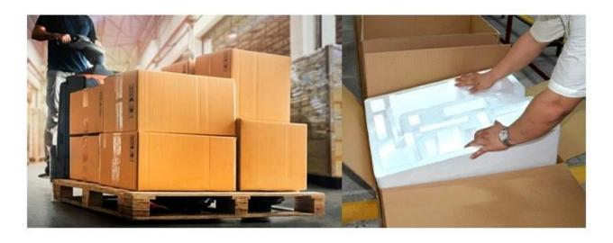
Cardboard Box Packing: Standard export boxes with internal cushioning of pearl cotton to ensure safe transportation of goods. Warning signs for proper box placement and waterproof bags inside.
