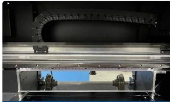
High quality drag chain, it is rub-resistance which greatly improves the service life.
